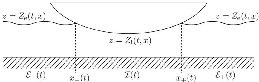
FIGURE 2. Waves interacting with a floating body
