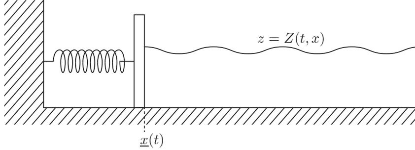
FIGURE 1. Waves interacting with a lateral piston
