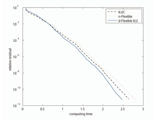
Figure 2: Example 2 - Convergence behavior of residual norm vs computation time,  $p = 80$
